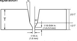
Wall thickness >3/4 in. (>20mm)
